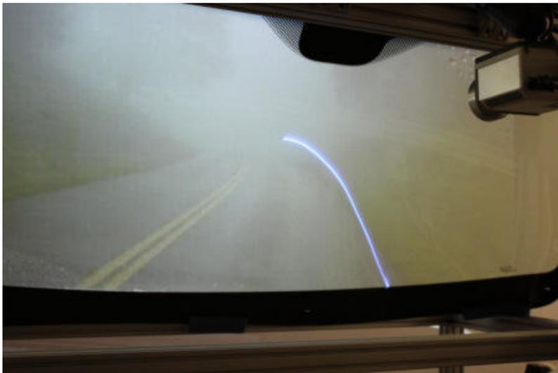
Researchers at General Motors R&D labs in Warren, MI, are working on an enhanced vision system. Various elements, including patent-pending technology from GM as well as patented technology from California-based **SuperImaging**, can effectively highlight on the windshield the road's edge during foggy weather.
